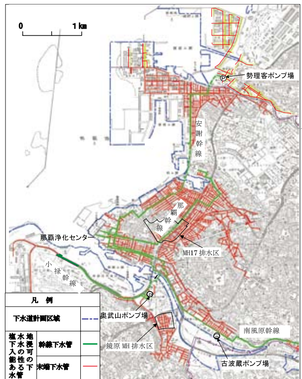
Fig.14 塩水地下水浸入の可能性のある下水管の分布状況 Distribution of sewer pipes having possibility of saline groundwater infiltration
