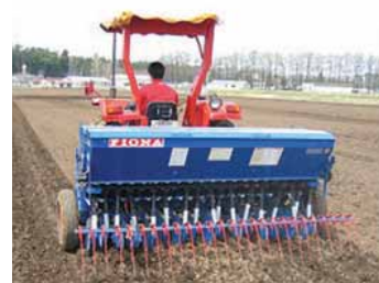
Direct seeding of paddy rice with a grain drill on an upland field.
