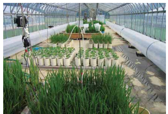
Temperature gradient chamber for research on the effects of interactions of temperature and CO 2 concentration on crops.
