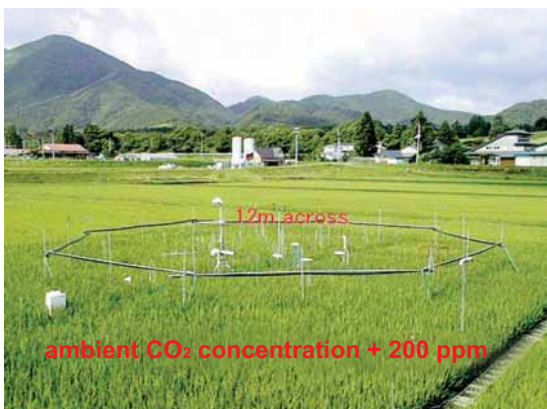
Free-air CO 2 enrichment (FACE) experiment at Shizukuishi, Iwate, as part of research on the effects of elevated CO 2 on rice growth and paddy ecosystems.
