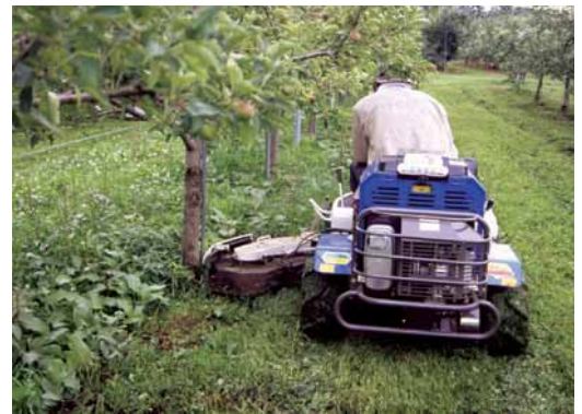
Weed control alternative to herbicide use: weeding the under-canopy of an apple tree by riding type mower.
