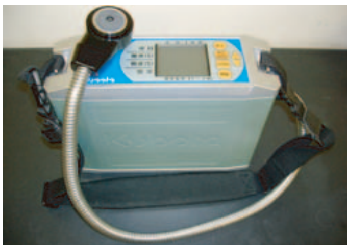
Photo.2 A portable near infrared spectrophotometer (Kubota K-BA100, Japan)
