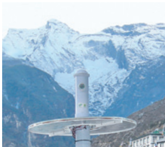
A Field Server working in Himalaya with a solar panel.
