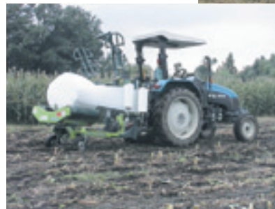
Self-propelled harvesting baler equipped with the attachment for forage rice
