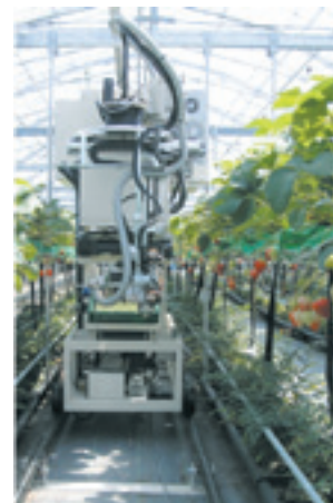
Development of a robot strawberry harvester
