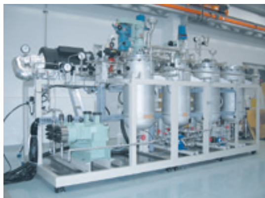
Supercritical methane-type STING-BDF manufacturing equipment
