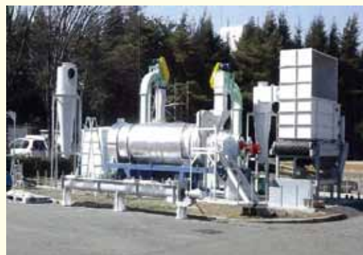
Equipment to stabilize and reduce volume of biomass contaminated with radioactive cesium by pelletizing
