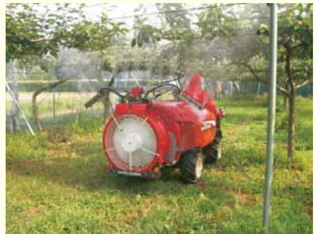
Less-drift orchard sprayer with less noise
