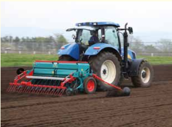
Dry seeding rice cultivation system using a high-efficiency grain drill that can be used for both rice and wheat
