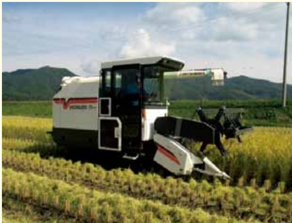
Compact general purpose combine harvester which is capable of being loaded on a 4t truckload truck and being used on narrow farm roads or farm land with no land readjustments
