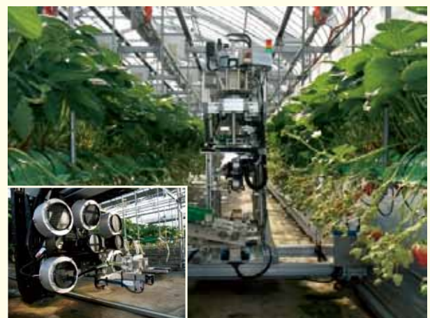
Strawberry harvesting robot which harvests only ripe strawberries by image processing with LED lighting and CCD cameras
