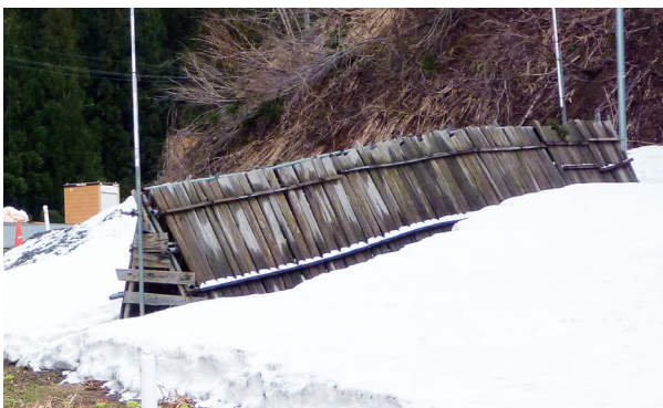
Fig.1 地表伸縮計の雪囲いの例 (七五三掛地区) Example of a shield to protect a surface extensometer from snow
