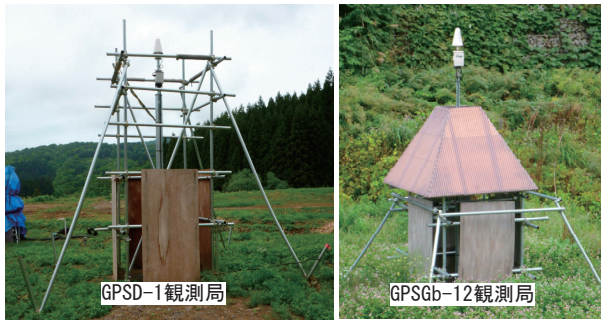
Fig.3 七五三掛地区におけるGPS観測局の例 Examples of GPS observation stations in the Shimekake district
