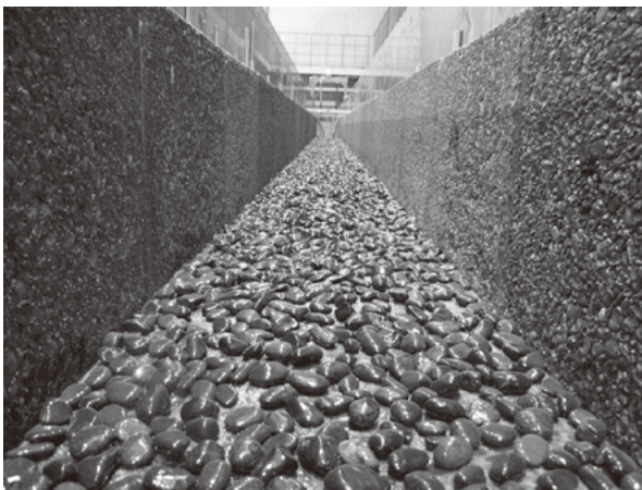
Fig. 1 模擬摩擦水路への礫設置状況 Installation of gravel to experimental channel
