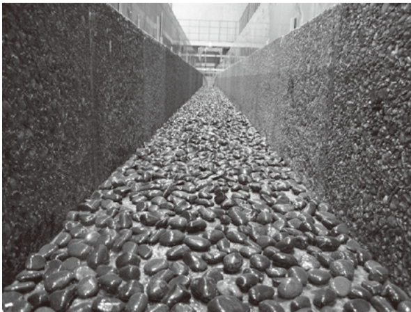
Fig. 1 模擬摩擦水路への礫設置状況 Installation of gravel to experimental channel
