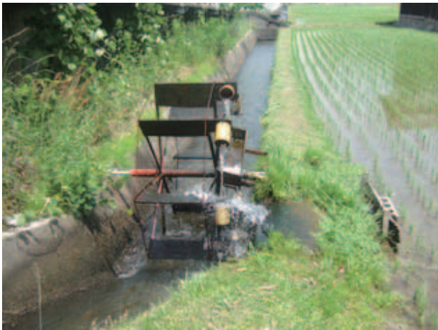
Fig. 38 上林地区の揚水水車の一例 (鉄製) Irrigation Water Wheel in Uchayashi district
