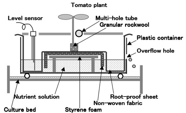
Fig. 4-3 Wet-sheet culture (WSC) system for the cultivation of single-truss tomato.
