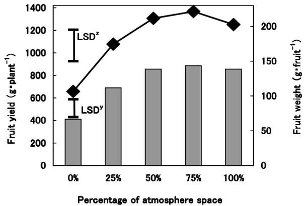
Fig. 4-5 Effects of atmosphere/solution space ratios in the root-zone on fruit yield and weight of single-truss tomato. ■, fruit yield; ◆, fruit weight. Vertical bars represent LSD at P=0.05. <sup>z</sup>LSD on fruit weight. <sup>y</sup>LSD on fruit yield.
