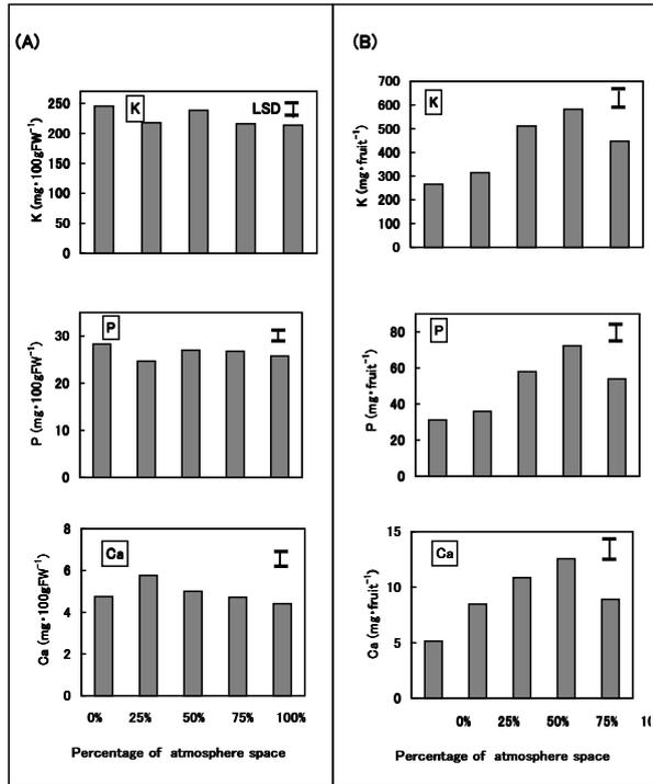
Fig. 4-6 Effects of atmosphere/solution space ratios in the root-zone on mineral contents of tomato fruit. A, fresh weight basis; B, whole fruit basis. Vertical bars represent LSD at  $P=0.05$  ( $n=21$ ).
