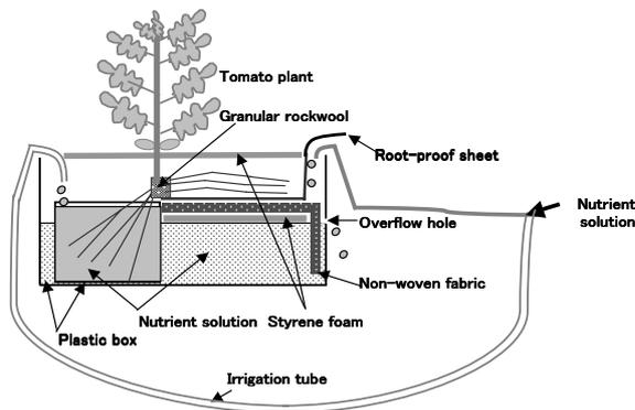
Fig. 4-1 Schematic diagrams of the experimental divided root culture system for the feeding of <sup>15</sup>N-labelled potassium nitrate to different parts of the tomato roots.
