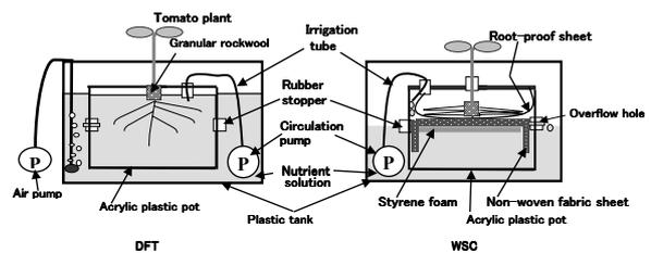
Fig. 2-7 Tomato seedlings were raised in two hydroponic systems, deep flow technique (DFT, left figure) and wet-sheet culture (WSC, right figure).
