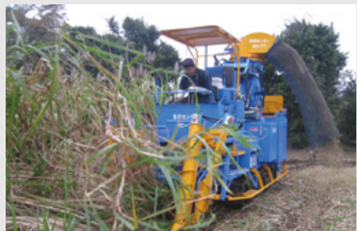
Small-size Sugarcane Harvester with High Chopping Performance
