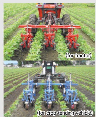
Disk-type Cultivator-Ridger A disk-type cultivator-ridger that suits to wet soil. (Commercialized)
