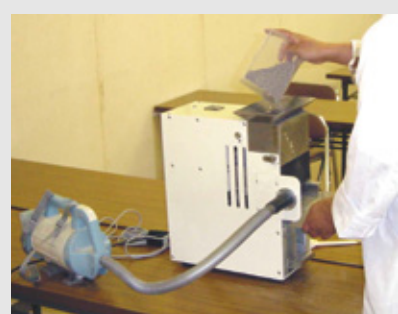
Soil Crusher-sieve A machine that crushes and sieves the dried sample soil for soil analysis (Commercialized)
