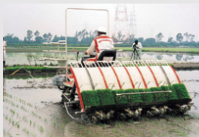
Field Performance Test of Rice Transplanter
