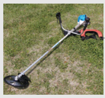
Low Vibration Bush Cutter The bush cutter with 30-40 % lower hand-transmitted vibration was developed for the purpose of preventing vibration disorders. (Commercialized)
