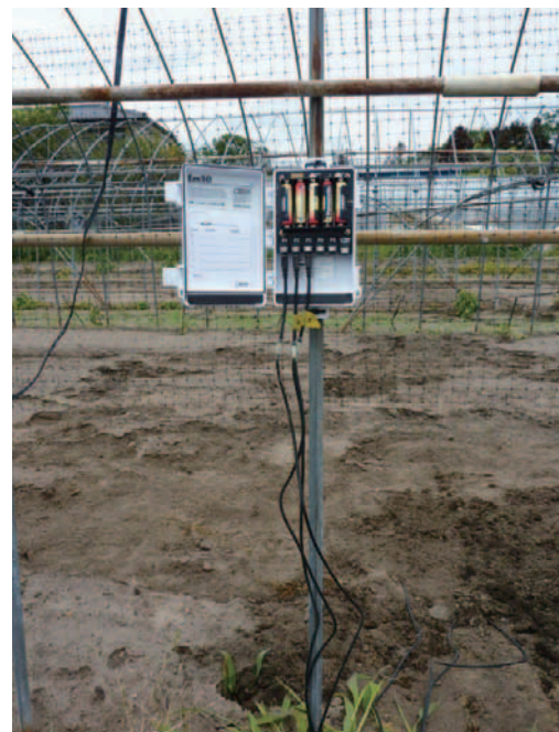
Fig. 4 データロガーによる観測 Field measurement by using data logger and dielectric soil moisture sensors
