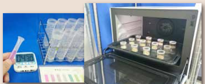
Rapid and simple soil testing method for available nitrogen in air-dried paddy soil
