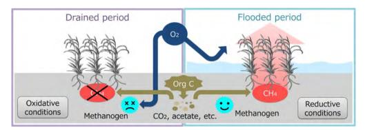
Fig. 1. Schematic representation of mechanisms underlying CH<sub>4</sub> emission from paddy soil.
