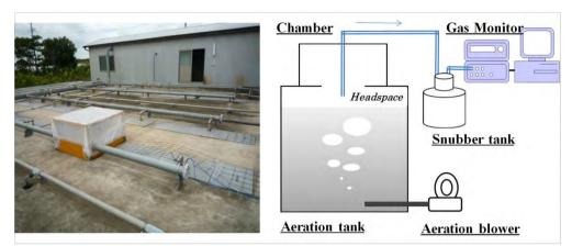
Fig. 3. System for measuring greenhouse gases from wastewater treatment plants.
