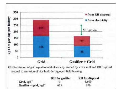
Fig. 4. Emission from 8 t h<sup>-1</sup> rice milling factory.
