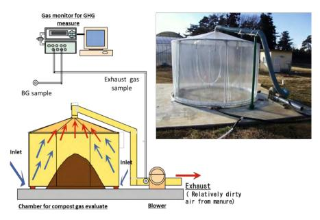
Fig. 1. System for measuring greenhouse gases from composting.
