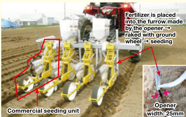
Cultivation of direct-seeded onion for processing use with the aim of shortening working hours (photo shows simultaneous fertilizing/seeding device that can apply phosphate fertilizer in advance just under the seeding depth)
