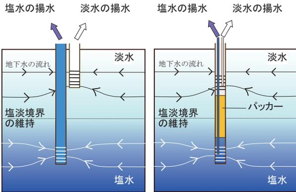
Fig.2 二重揚水手法 (左: 2孔式, 右: 単孔式) Scavenger/production well coupling
