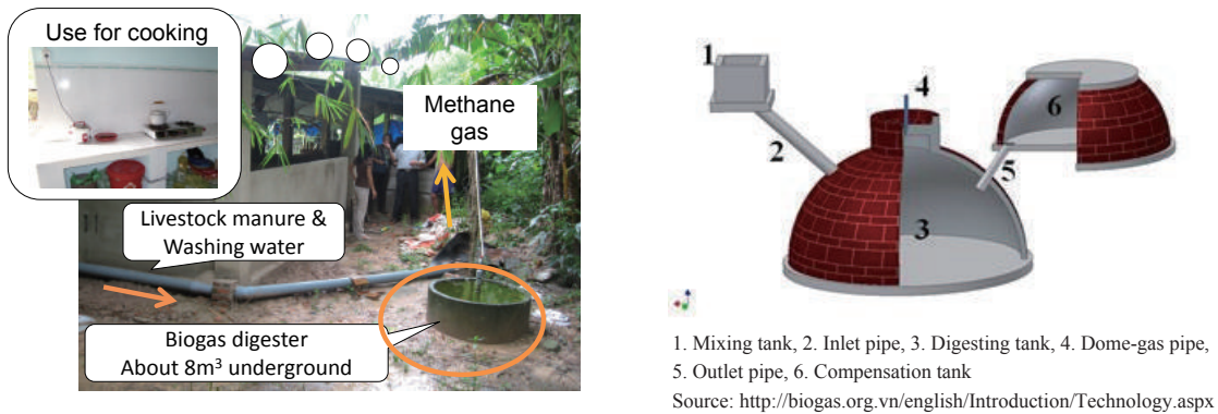
Fig. 1 Fixed dome type of household biogas digester
