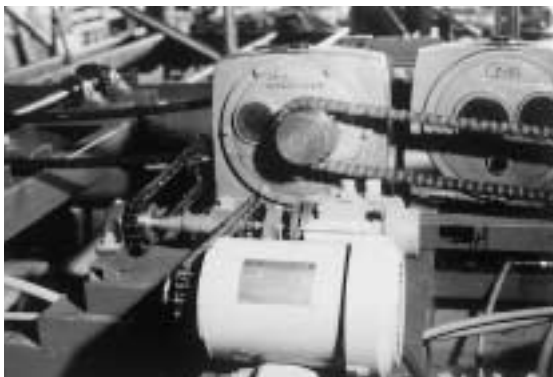
写真 20 作業装置昇降用モータと減速機 Photo 20 Motor and reduction gear for up and down movement of working device
