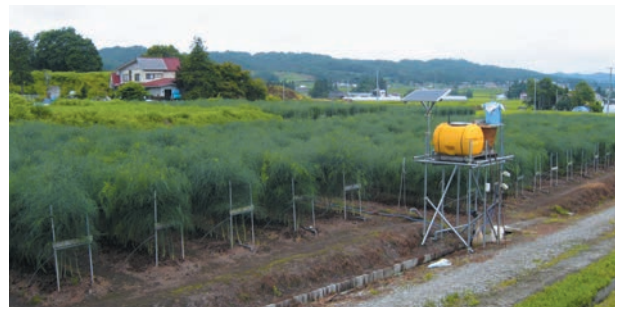
A solar radiation-dependent drip irrigation system that facilitates labor-saving in irrigation and fertilization (Figure: Asparagus field)
